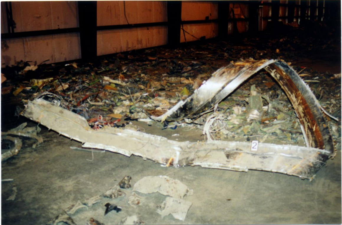
Photo 8. No. 2 engine fan containment case.
