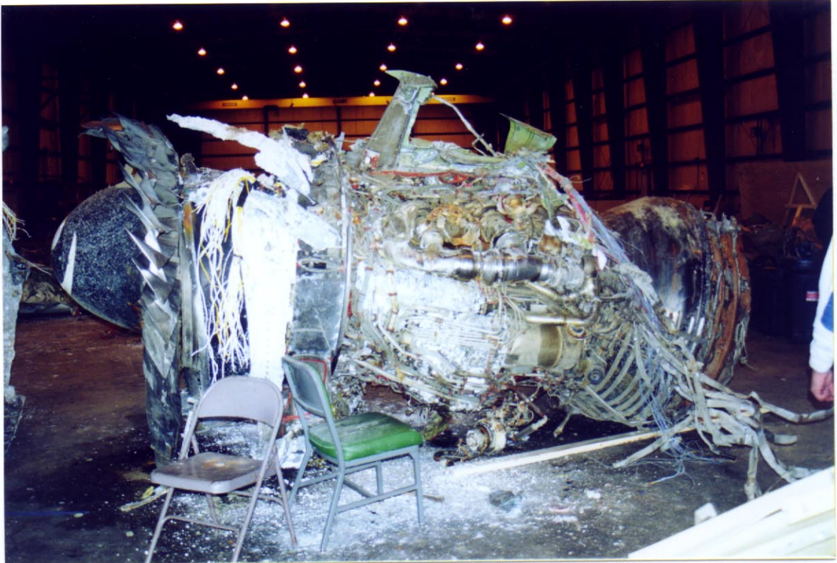
Photo 3. View of left side of No. 1 engine.
