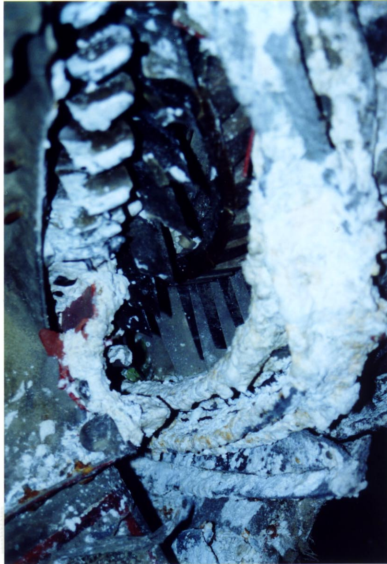
Photo 5. Close up view of LPC disk and blades visible through separated flange.
