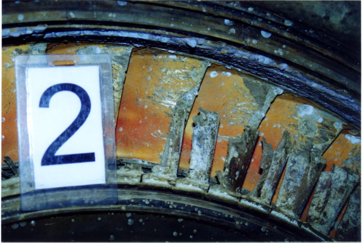
Photo 21. Closeup view of No. 2 engine broken HPT blades and intact vanes.
