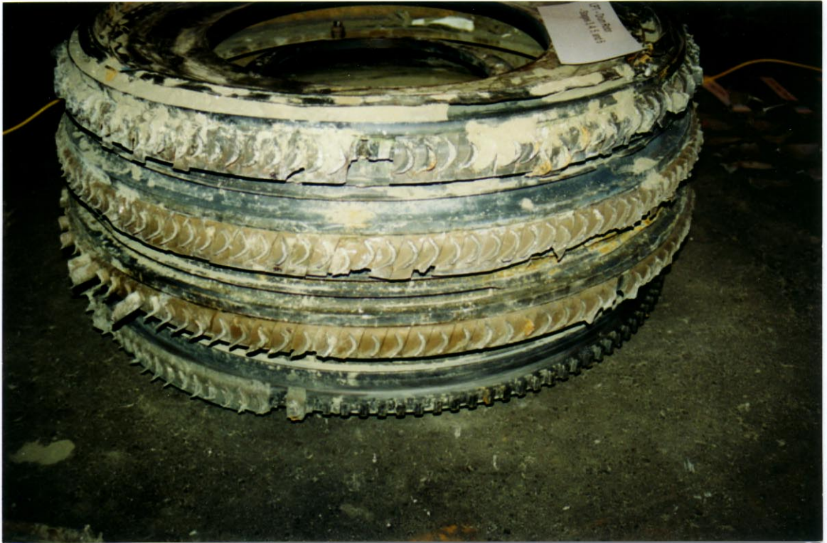
Photo 22. View of No. 2 engine LPT rotor with LPT blades broken off.
