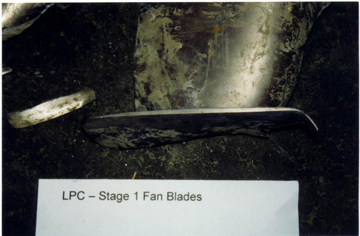
Photo 11. Closeup view No. 2 engine fan blade tips showing no rub marks.
