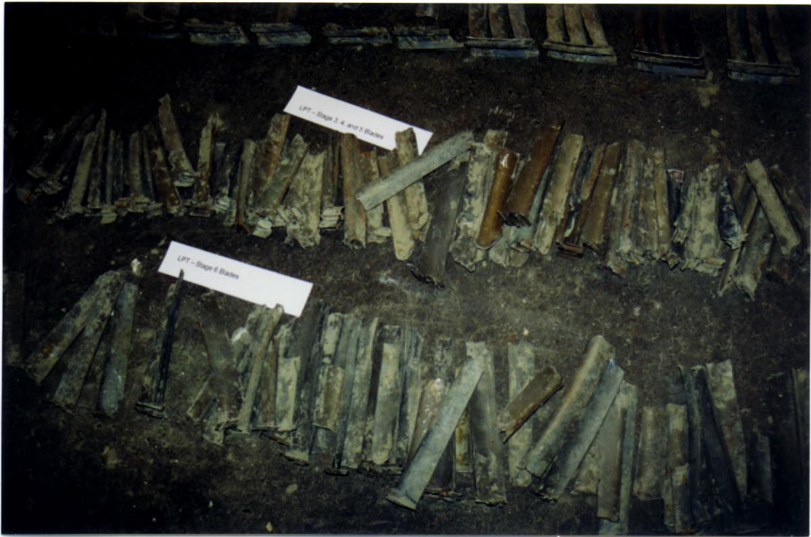
Photo 24. No. 2 engine LPT blades showing full length airfoils.
