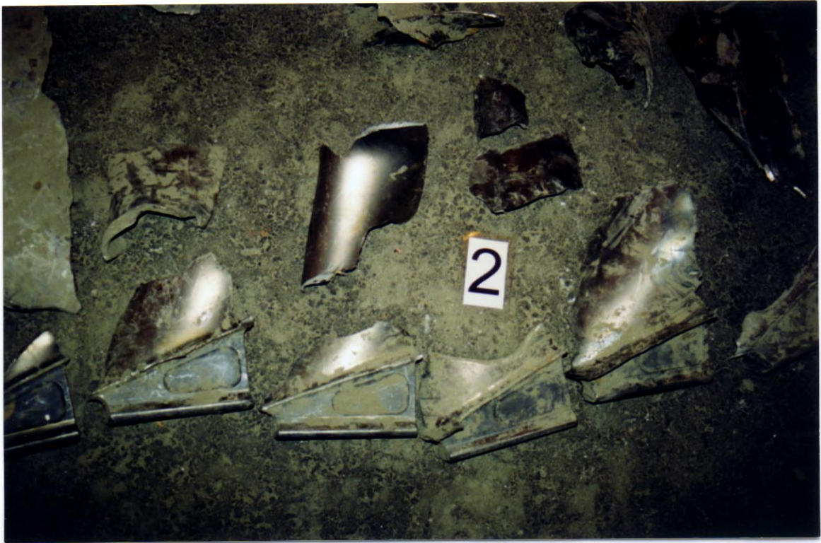
Photo 10. Pieces of No. 2 engine fan blades.
