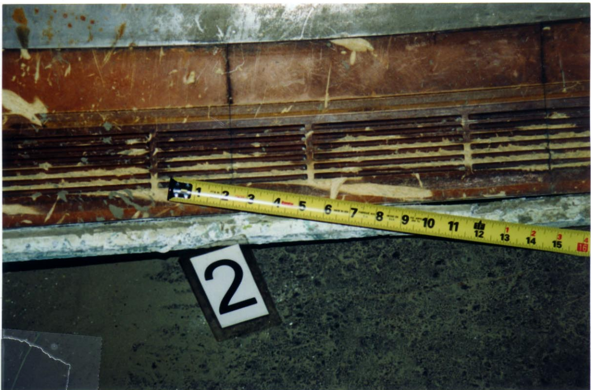
Photo 9. Closeup of No. 2 engine fan rubstrip showing imprints of fan blade tips.
