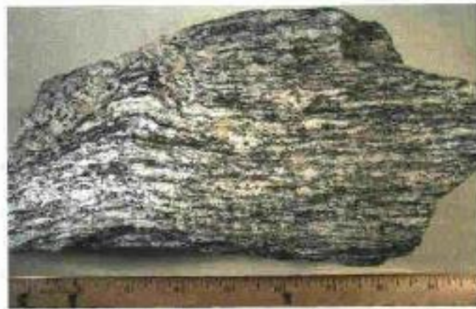
The laminar structure is evident in this specimen of biotite schist (Courtesy of Darryl Maddox, Amarillo College)
